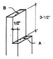
Make four 3 foot square frames from the lap jointed 2x4s. Use one pressure treated 2x4 on each frame. Put enough construction adhesive to fill the gaps when the lap joints are screwed together. Fasten each joint with four screws.
