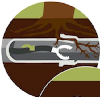
◀ Pipe with **ROOT INTRUSION** being cleaned with a cable fitted with a root-cutting blade.
