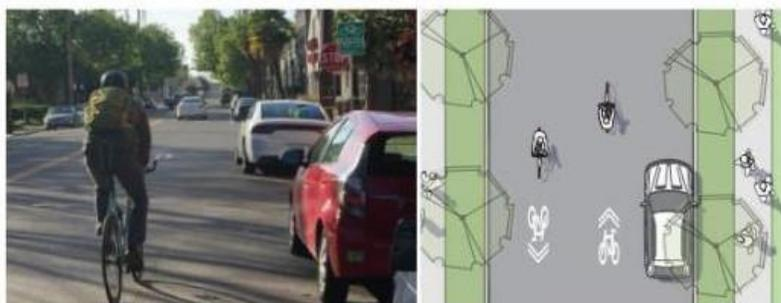
**Class IV Separated Bikeway: a bikeway in the roadway separated from vehicle traffic by physical barriers.**
