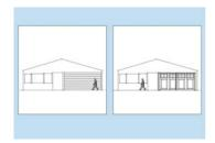
C3: Articulate garage doors and separate two-car garage doors into two one car garage doors.
