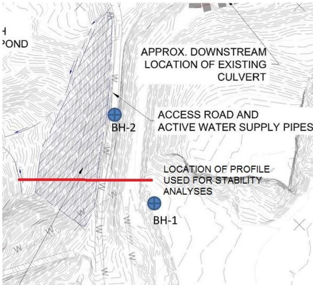
**Figure C-6: Approximate Locations of Geotechnical Borings (BH) and Profile for Stability Analysis.**
