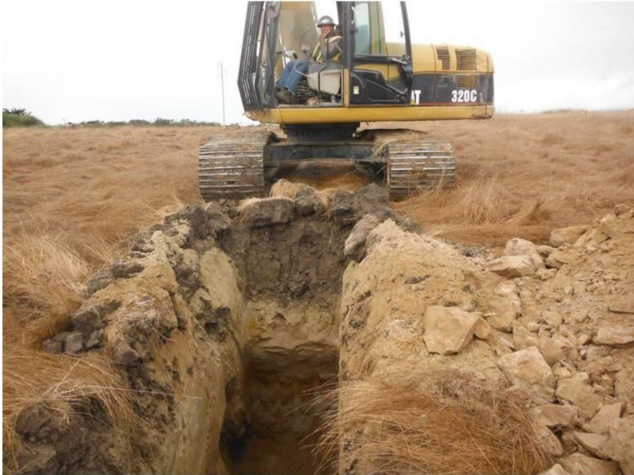
**Figure C-5: Test Pit 25 example of excavation in weathered rock (Mudstone). View toward west.**
