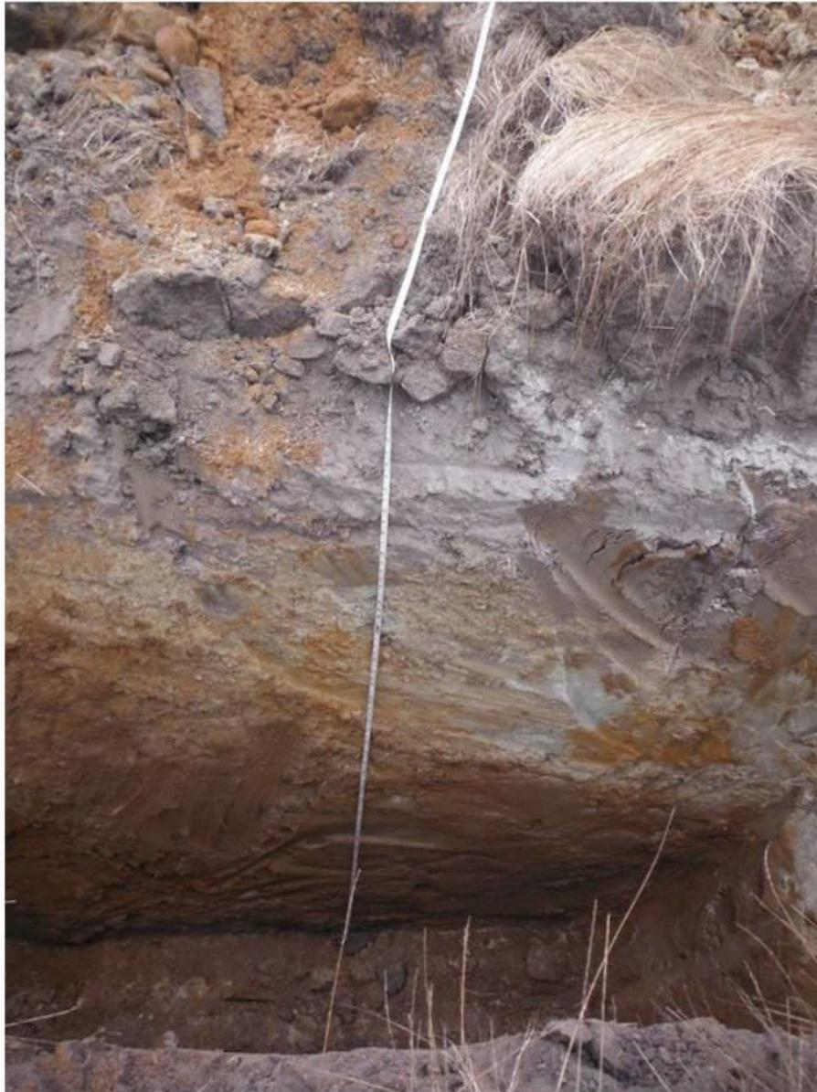
**Figure C-4: Test Pit 24 example of cut slope stand-up in excavated topsoil through weathered rock.**
