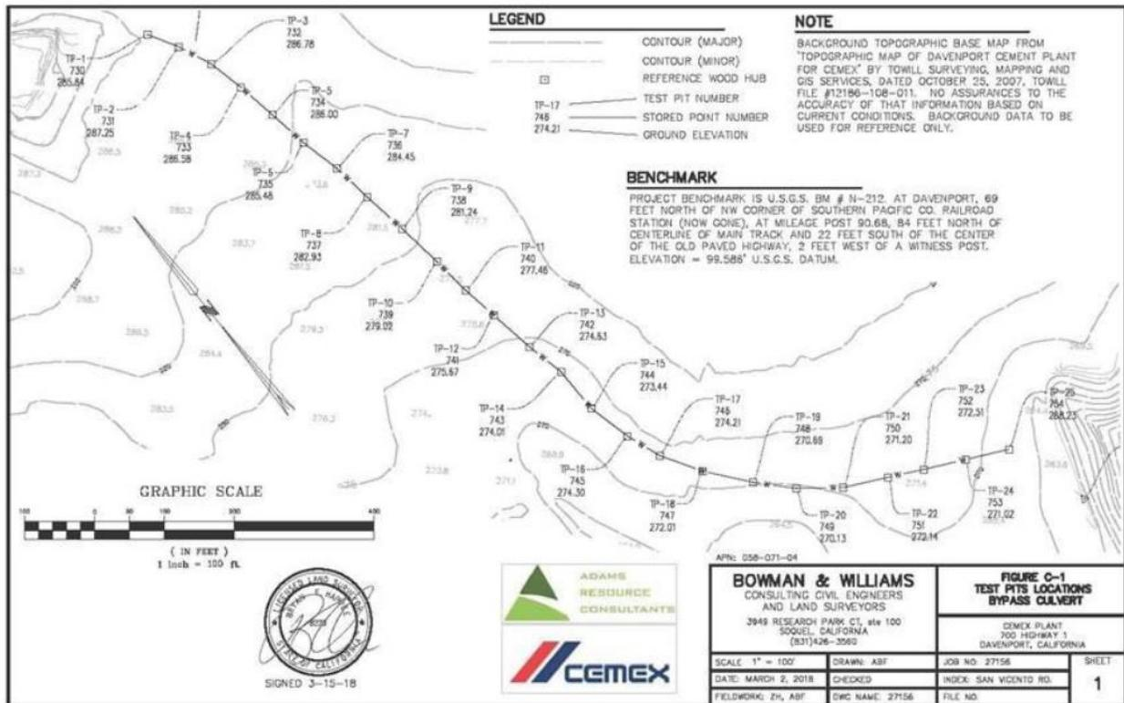
**Figure C-1: Survey Map Showing Test Pit locations near the Bypass Pipeline alignment.**
