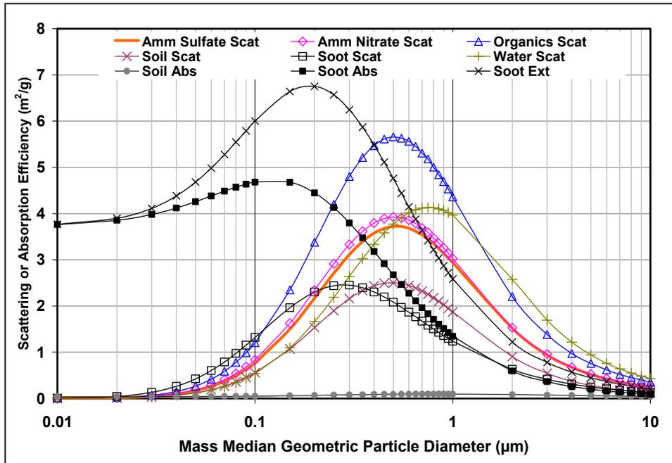
Figure 3-2 Particle scattering efficiencies as a function of size distribution for different particle compositions (Watson, 2002). The geological scattering efficiency (Soil Scat) is lower than that for other PM chemical components and decreases rapidly with particle size.
