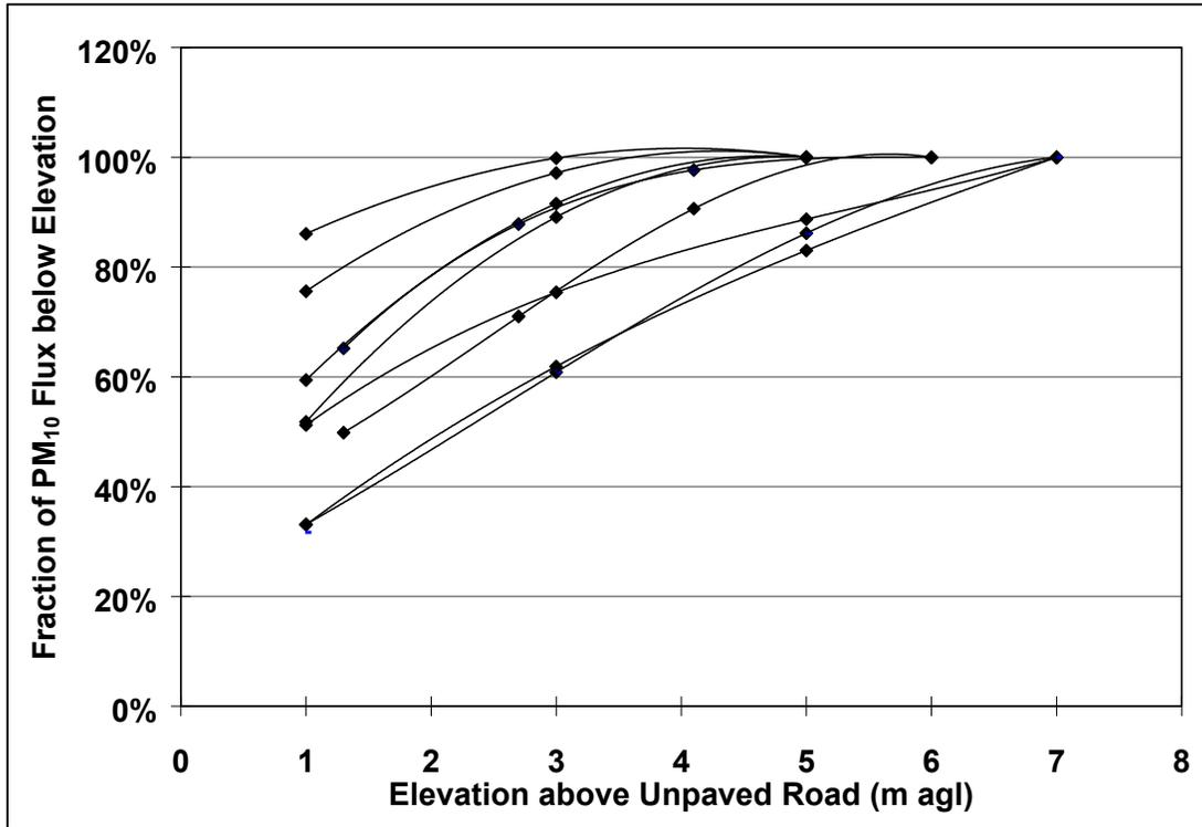
Figure 2-4. Cumulative horizontal PM<sub>10</sub> flux at different downwind elevations above different unpaved roads (Watson et al., 2000).
