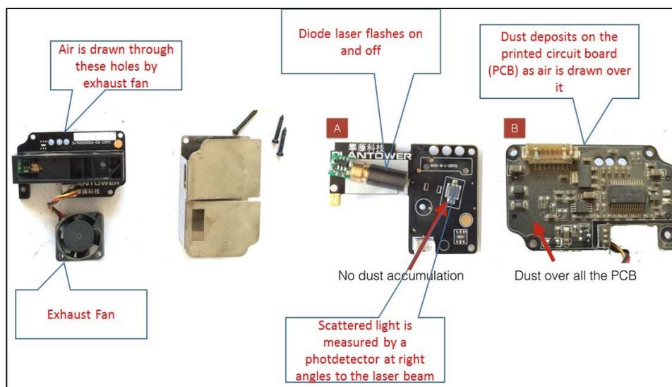
Figure 3-6. Internal configuration of the Plantower 5003 particle sensor (<https://aqicn.org/sensor/pms5003-7003>).
