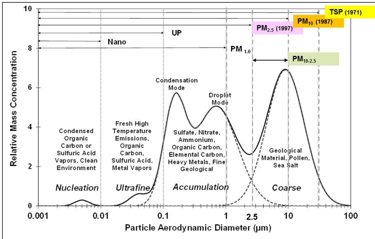
Figure 2-3. Illustration of different modes in a typical atmospheric particle size distribution. Nucleation and Aitken modes often overlap. Note that the tail (dotted line) of the accumulation mode penetrates into sizes  $<0.1 \mu\text{m}$ , as does the coarse mode into the accumulation mode. Sources and processes that affect each mode are indicated. Based on Chow (1995) and Watson (2002). The years in which U.S. ambient air quality standards for each size indicator are noted parenthetically.
