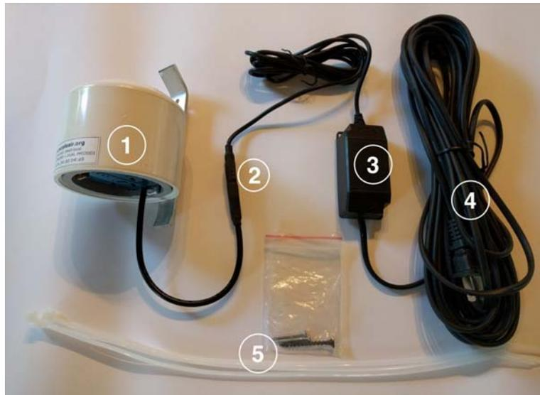
Figure 3-3. The PurpleAir (2019) microsensor that is being used throughout California and other states for citizen science and implementation of AB 617 (Garcia, 2017). The package includes the sensor in protective cover (1), micro-USB cable (2), 5V power supply (3), 120 V line cord (4), and mounting screw and zip-ties.
