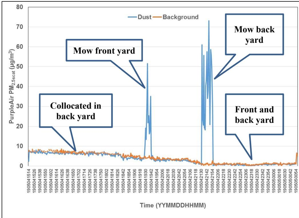
Figure 3-8. Example of dust detection over background. The Dust sensor was placed on a lawnmower after being collocated with the Background sensor. Dust generated by the mower is evident over background. The mower remained in the front yard, then was used to mow the backyard and parked next to the Background monitor.
