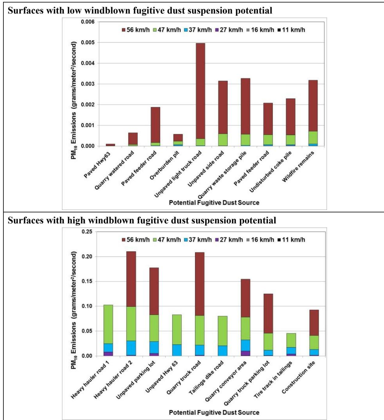
Figure 2-2. Windblown fugitive dust suspension potential measured with a portable wind tunnel in and around industrial operations in Canada’s oil sands region of northern Alberta (Wang et al., 2015). The difference in suspension potential depends more on the frequency and intensity of surface disturbances rather than on the type of surface. It is also evident that higher wind speeds increase the reservoir size in addition to adding energy to the suspension process.
