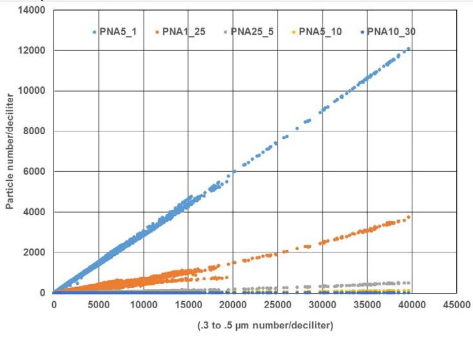
Figure 3-7. Comparison among five collocated PurpleAir sensors for the reported size fractions compared with the smallest size fractions. The manufacturers have apparently included constant multipliers to estimate the different size fractions from the light scattering output of the sensor.
