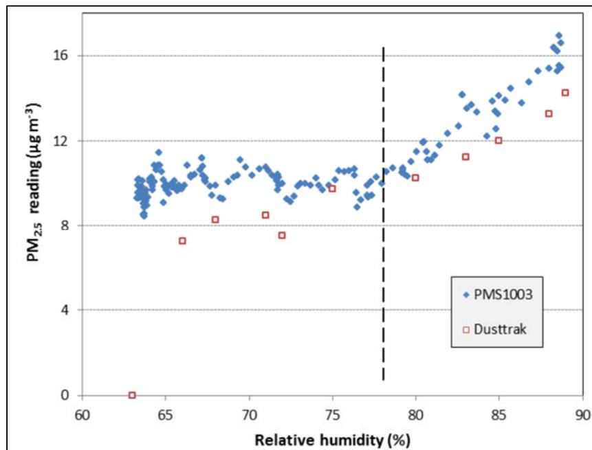
Figure 3-9. Relationship between Plantower reading and relative humidity in a controlled laboratory experiment (Jayaratne et al., 2018). The same effect is demonstrated for the DustTrak (Wang et al., 2009), another light scattering detector.
