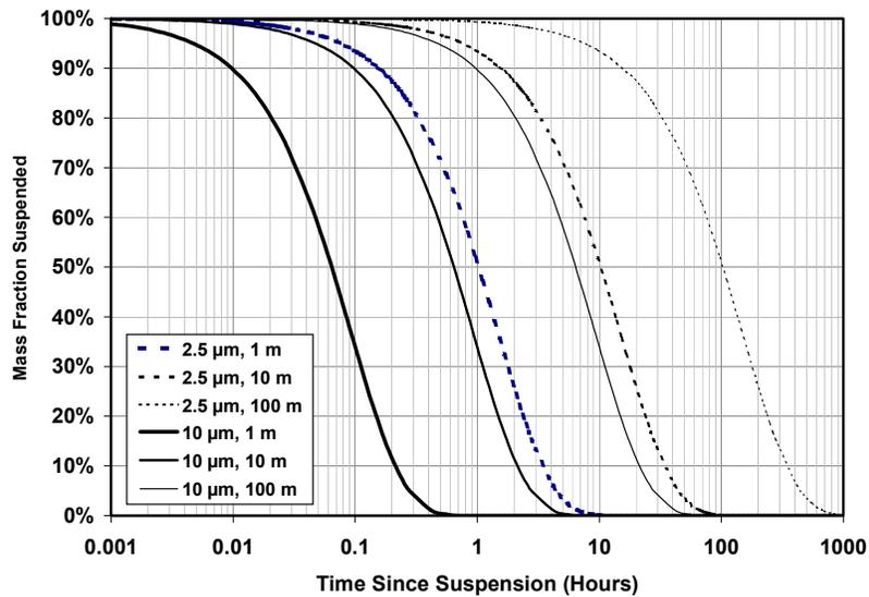
Figure 2-5. Attenuation of mass concentrations for 2.5 and 10  $\mu$ m aerodynamic diameter particles with time and vertical mixing height (1 to 100 m). This assumes a stirred tank model (Hinds, 1999) in which particles are homogeneously redistributed throughout the mixed layer at each time step and gravitational settling velocities.
