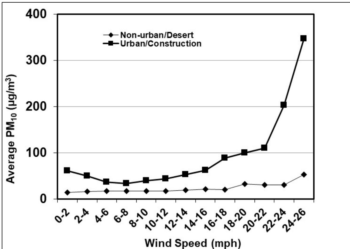
Figure 2-1. Average PM<sub>10</sub> concentrations for different wind speed categories (mph=miles per hour) measured near a graded construction site and undisturbed desert near Las Vegas, NV (Watson et al., 2000) with a beta attenuation monitor (BAM).
