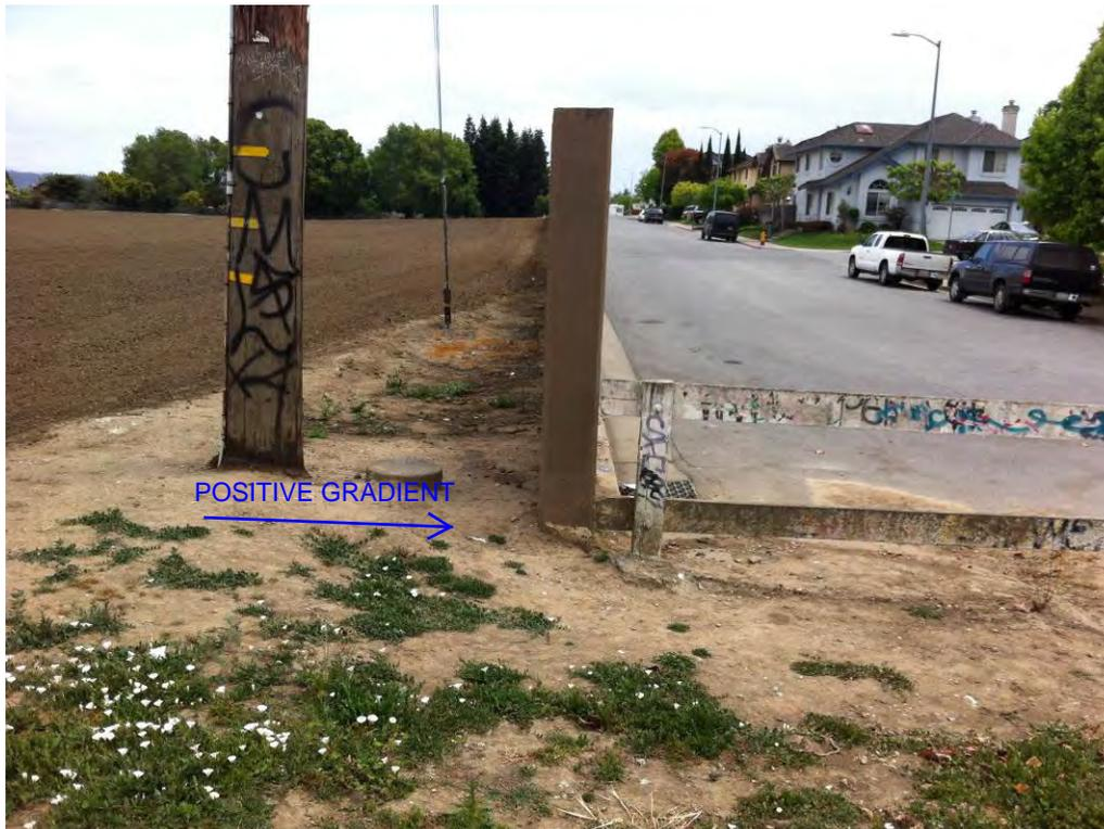
**Figure 2: Agricultural Fields at Higher Elevation than the Inlets Brewington Avenue**
